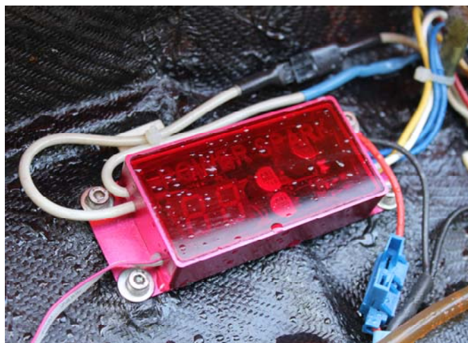
Waterproof POWER SPARK system left corner: programming cable (special development version)
